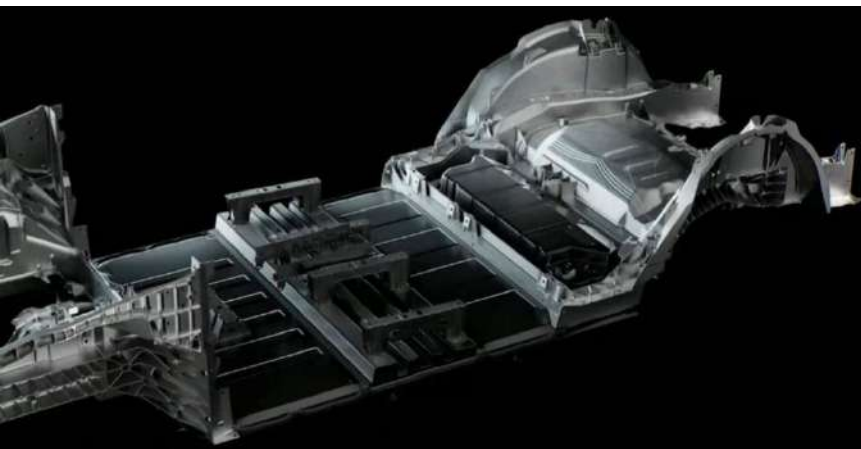
大型壓鑄一體化汽車結構件 Die-casted Giant Size Integrated Automotive Structural Parts
